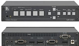
The VP-461 is a high-quality presentation switcher and scaler with PIP for computer graphics, HDMI and DisplayPort signals. It scales the video, embeds the audio and outputs the signal to the HDMI output, as well as to the computer graphics video output together with an unbalanced audio output
